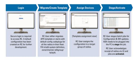
Figure 1: APX N70 Provisioning via Radio Central
